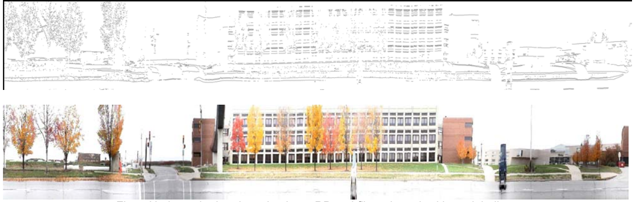
Fig. 4 Horizontal edge detection in an RP and filtered result with straight lines
