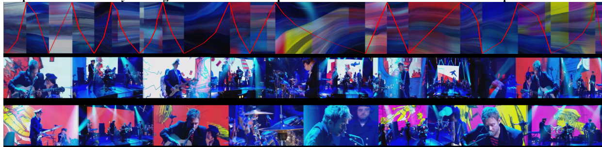
Figure 9. Consecutive profiles of a concert video with simultaneous zoom and pan. (Top) Vertically condensed flow graphs. (Lower) Profile cut from the trajectory in the flow graph above. The profile is temporally scaled up.
