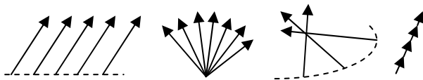
Fig. 3 Typical camera works with zoom, translation and rotation. The arrows indicate the movement of camera axis, and their lengths correspond to the camera focal lengths. (a) Translation, (b) pan/tilt, (c) around-object rotation, (d) zoom in/out.
