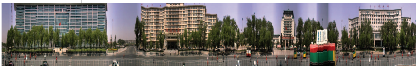
Figure 5. A segment of route panorama generated from a video taken on a bus (before removing shaking components).
