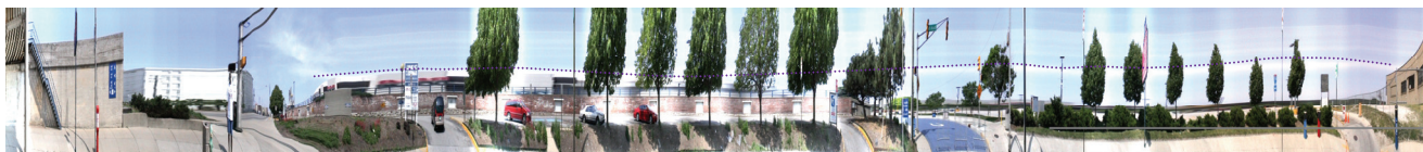
Figure 2: A section of route panorama, RP(t,y) , in which a piece of cloud at infinity is projected as a trace (indicated by dotted curve) over two blocks. It reflects the waving of camera as a “lighthouse” feature.
