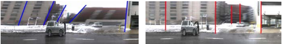
Fig. 6. Slanted vertical rims in the scene tunnel if the sampling line is not precisely aligned with the projection of a vertical line. (a) Declined edges due to imperfect alignment of the pixel line. (b) A precisely set sampling line generates a good shape of vertical lines.
