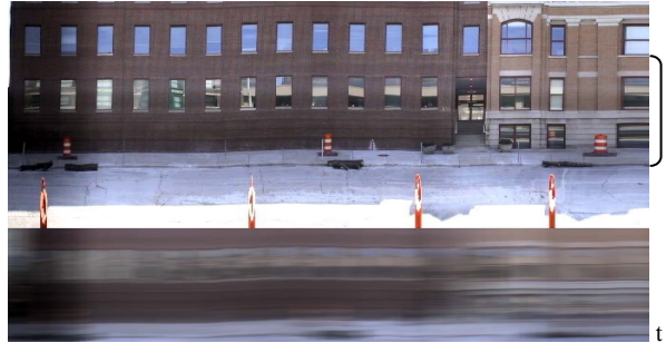
Fig. 6 Horizontally integrated image for motion detection. (a) Route panorama. (b) Condensed image in which traces are continuous on repetitive windows.
