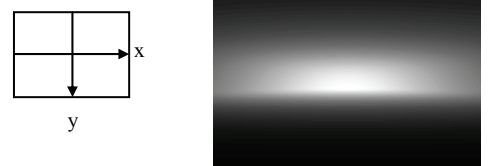
Fig. 3. The probability of vehicle features p(x, y|C) in the image frame displayed in gray level.
