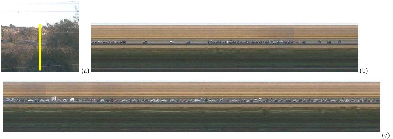
Figure 3 Detecting dynamic objects in real time. (a) Field of view with a sampling line intersecting a distant road. (b) A section of line sensor image with vehicles and their times of arrival. (c) Detected vehicles and the transmitted sections.
