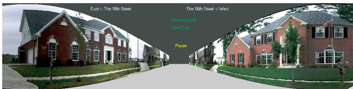
Figure 8. An opened form of the cylindrical surface dynamically displaying forward and side views.
