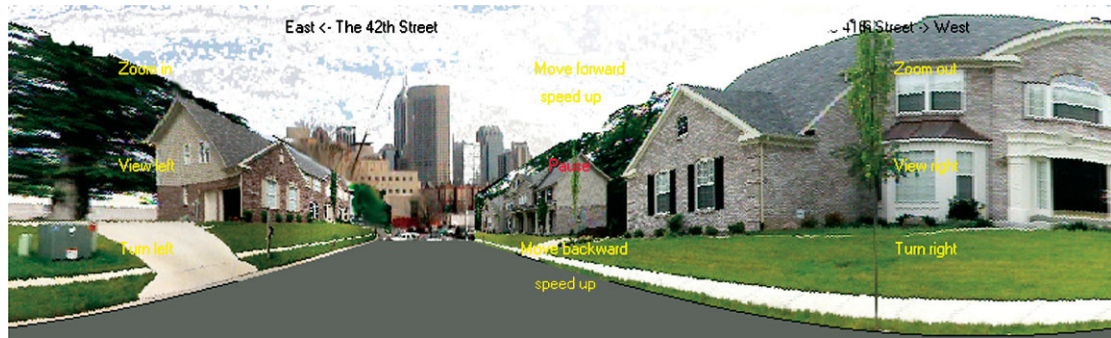
Figure 9. A panoramic traversing window dynamically displaying route scenes in an opened form of panoramic view. Traversing control is realized by mouse clicking in embedded sub-areas.
