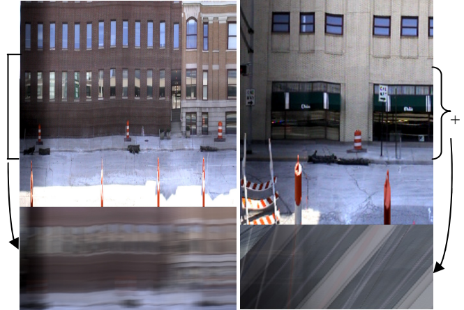
Figure 4 Examples of condensed image slice (right) and condensed motion trace (left) with range of summation.
