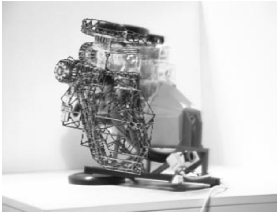
Figure 5.13: When the model is turned and its movements tracked, the graphics show the misalignment in the camera's z -direction.
