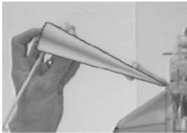
Figure 15: The model of a pointer is aligned with the physical pointing device by using the results of pointer and tracker calibration.
