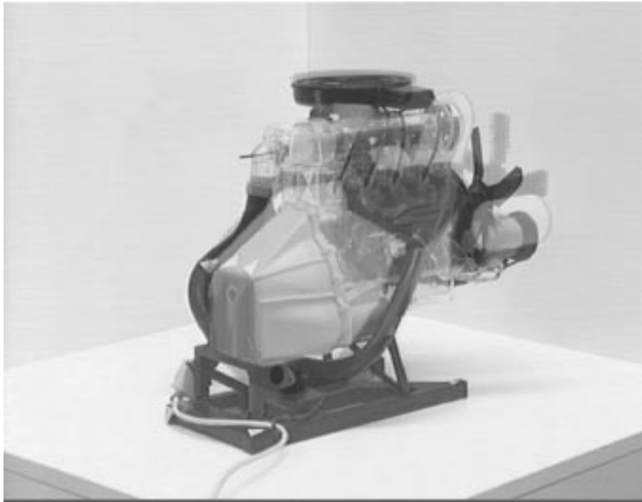
Figure 17: A shaded engine model registered to a real model engine using an image-based calibration. The geometric model is shaded in red, blue and yellow, before being overlaid on the plastic model.
