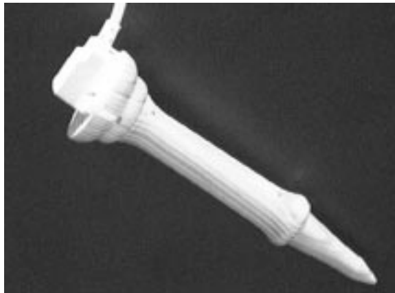
Figure 5: The pointer object consists of a wooden wand with a tracker receiver attached to the base and a tapered tip. The tip is considered the “hot-spot” during user interaction.
