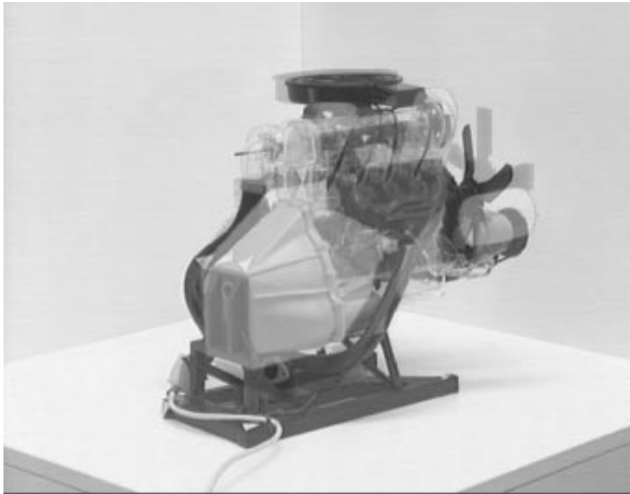
Figure 19: A shaded engine model registered to a real model engine using a pointer-based calibration.
