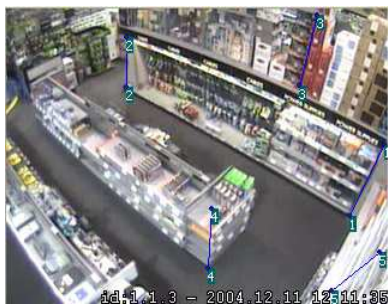
Figure 2: \mathbf{V}_Z can be found by manually marking two or more vertical straight lines
