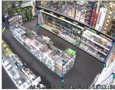
Figure 3: \mathbf{V}_Z can be found by manually marking two or more vertical straight lines
