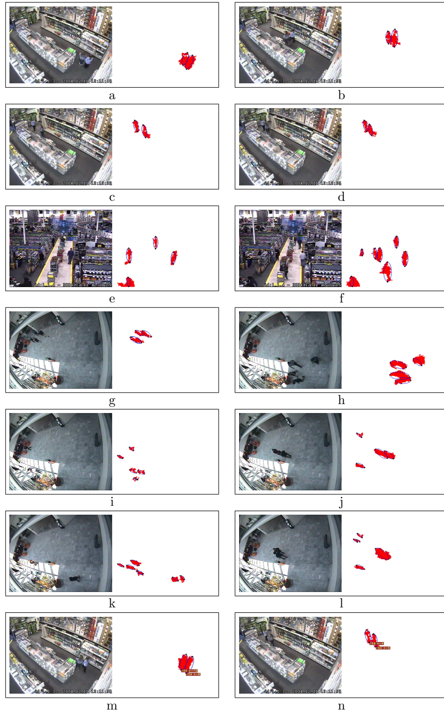
Figure 8: (a) - (l) Head candidates from test frames. Left image is the original frame. On the right image red represents foreground mask, small black dots indicate the locations of \mathbf{T}_i and \mathbf{B}_i ; blue ellipses are fitted with \mathbf{T}_i \mathbf{B}_i as the major axis; (m) and (n) Height detection: brown plates contain height mean and variance for each ellipse
