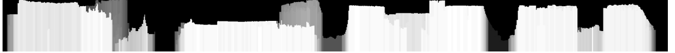
(a) Depth map of buildings from a camera path is predicted from LIDAR data (intensity is inversely proportional to the depth).
