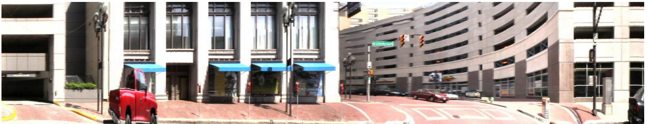
Figure 5 A segment of route panorama with front and side facades of buildings. The Plane of scanning is forward in about 45° from the camera moving direction.
